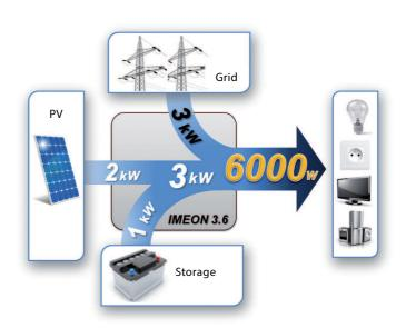
2kW of solar energy, 1kW of battery power and 3 kW from the grid for a total draw and output of 6kW. Thus, the installer does not need to modify the domestic electrical panel if it can provide energy less than or equal to 6kW.
