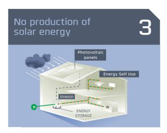
The batteries feed the domestic consumption needs. When needed, an eventual compliment of electricity is supplied by the public grid.
